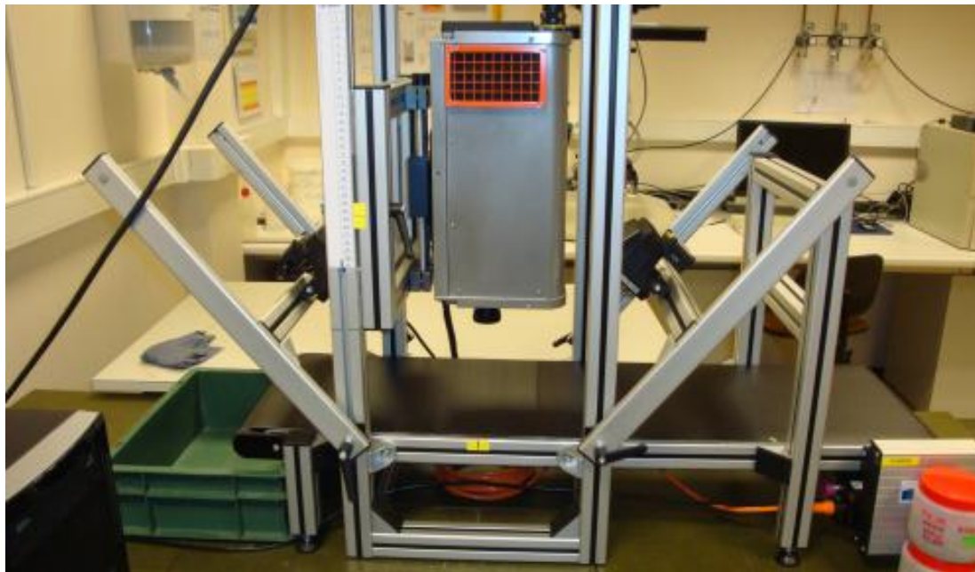
NIR line scan imaging system
