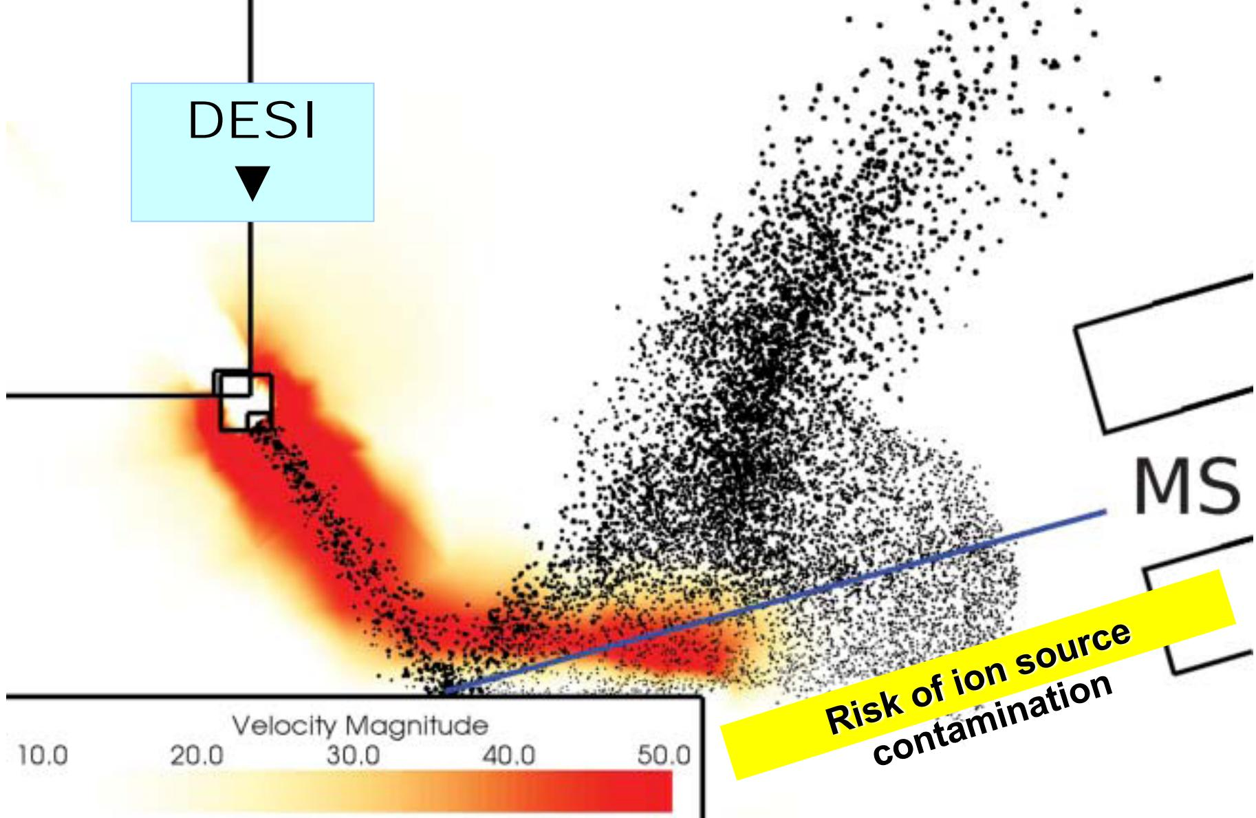
Spray and fluid velocity illustration. Droplets are black spheres eight times their actual size. Background color indicates velocity magnitude of surrounding fluid. The blue line shows the optimum collection angle from experiments ( $\sim 10^\circ$ )
