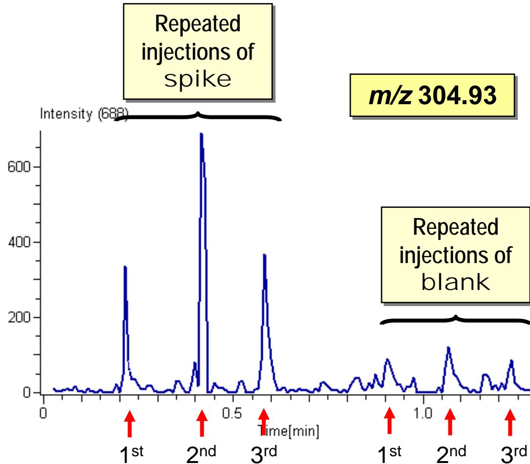
*Sample introduction variations compensated using an internal standard (TPP)*
