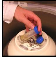
Centrifugation – 5 min, 11,000 rpm
