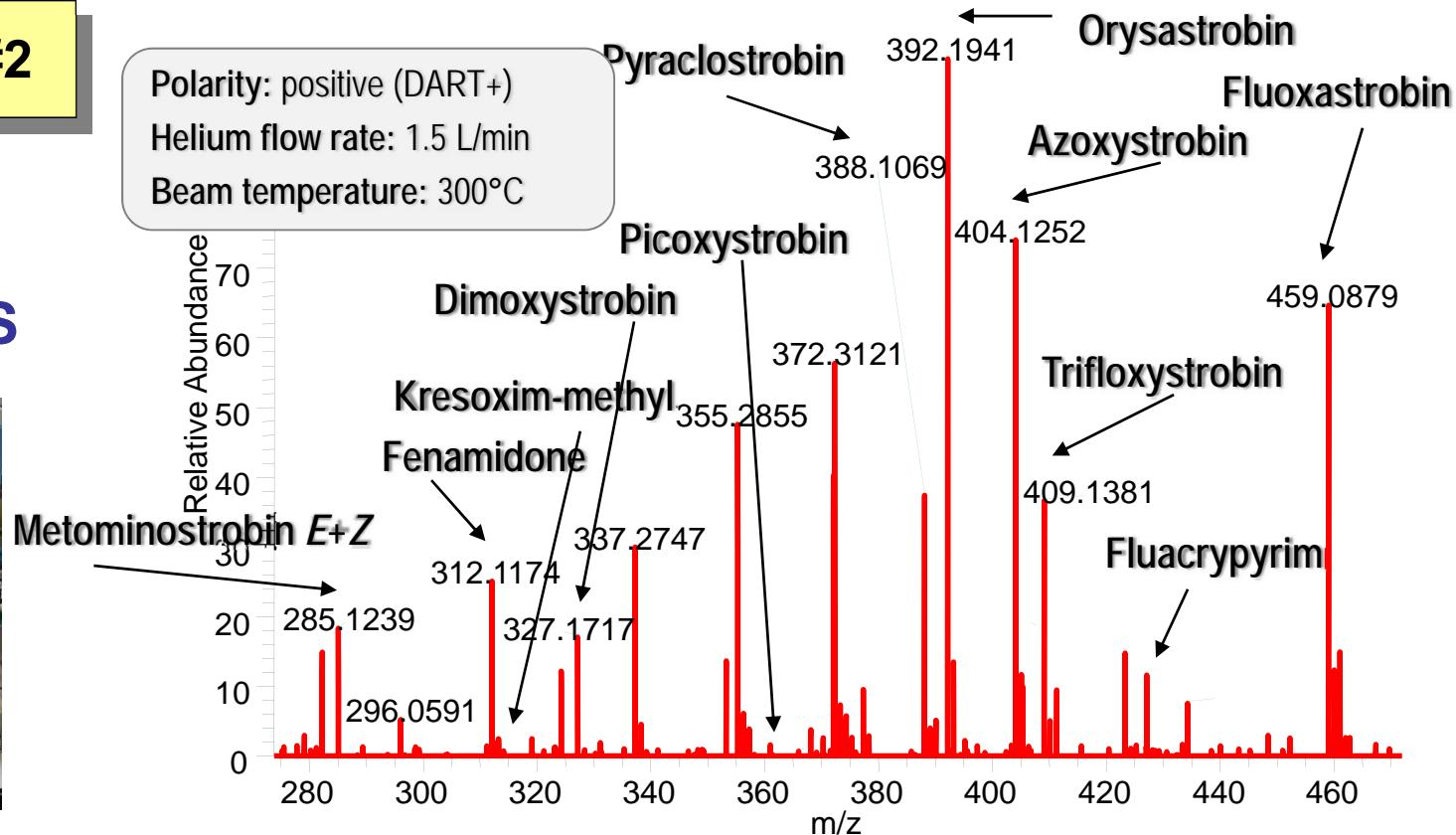
Purified (PSA, C18) QuEChERS extract (wheat) spiked with strobilurins at 1 mg/kg
