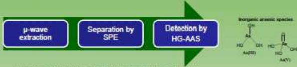
FIGURE 1. Principle of the MAE-SPE-HG-AAS approach for selective speciation analysis of inorganic arsenic.
