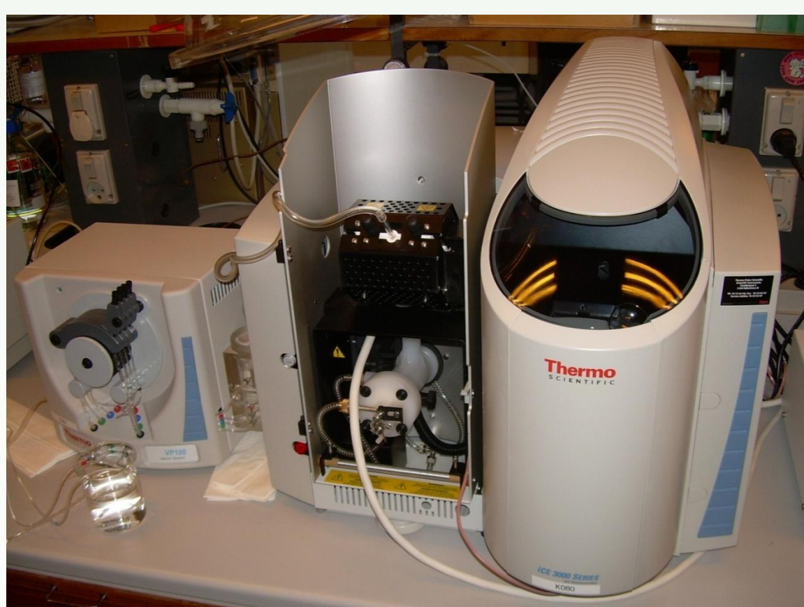
PICTURE 1. ICE 3300 AAS from Thermo Scientific with a VP100 for hydride generation system and an electrically heated cell.
