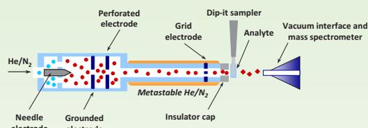
Figure 1: Scheme of DART ion source.
