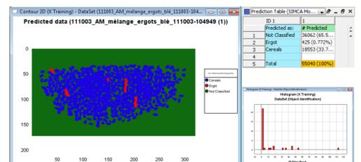
The first image shows the typical spectra for several cereals kernels and ergot bodies. The second image shows the prediction results of the SIMCA (Soft Independent Method of Class Analogy) model for an adulterated wheat sample on the tray. Wheat grains are in blue, ergot bodies in red and background in green. The number of pixels counted for each class of the model and the distribution of groups of pixels detected as ergot are also provided.
