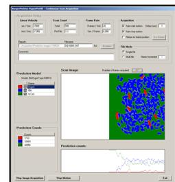
The first image shows the typical spectra for wheat kernels and ergot bodies. The second image shows the analytical parameters used and the on-line prediction results of the PLSDA (Partial Least Squares Discriminant Analysis) model for an adulterated wheat sample on the conveyor belt. Wheat grains are in blue, ergot bodies in red and background in green. The number of pixels counted for each class of the model is also provided.
