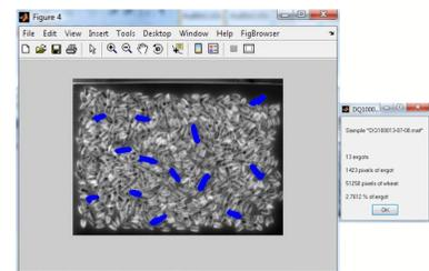
The first image shows the typical spectra for wheat kernels and ergot bodies. The second image shows the results of the prediction using a SVM (Support Vector Machine) discrimination model for a wheat sample adulterated with ergot. After applying the density-based clustering method (DBSCAN), wheat grains are in grey, ergot bodies in blue and background in black. The number of ergots and the number of pixels counted for each class of the model is also provided.
