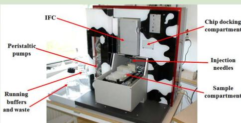
Figure 1: Biacore prototype multiplex biosensor
