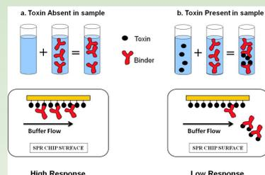
Figure 2: Schematic of SPR optical biosensor inhibition assay format
