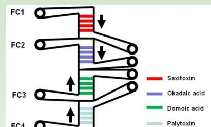
Figure 4: Schematic of chip surface with toxins immobilised as per flow cell of the instrument
