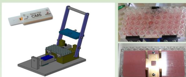
Figure 3: Chip surface immobilisation unit and upper and lower views of loading wells (x16 left and right) for immobilisation of components
