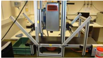
Figure 1: Image acquisition of cereals kernels using a line scan hyperspectral imaging system instrument.
