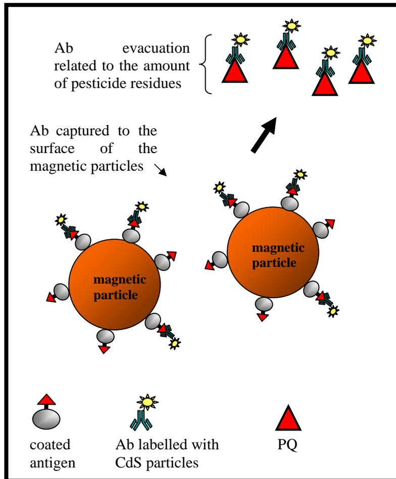
*Fig. 1. Electrochemical immunosensor reaction. An amount of the specific antibody is captured by the coated antigen. Likewise, the amount of Ab bound to the pesticide was evacuated. The amount of CdS particles is indirectly related to the PQ residues concentration.*
