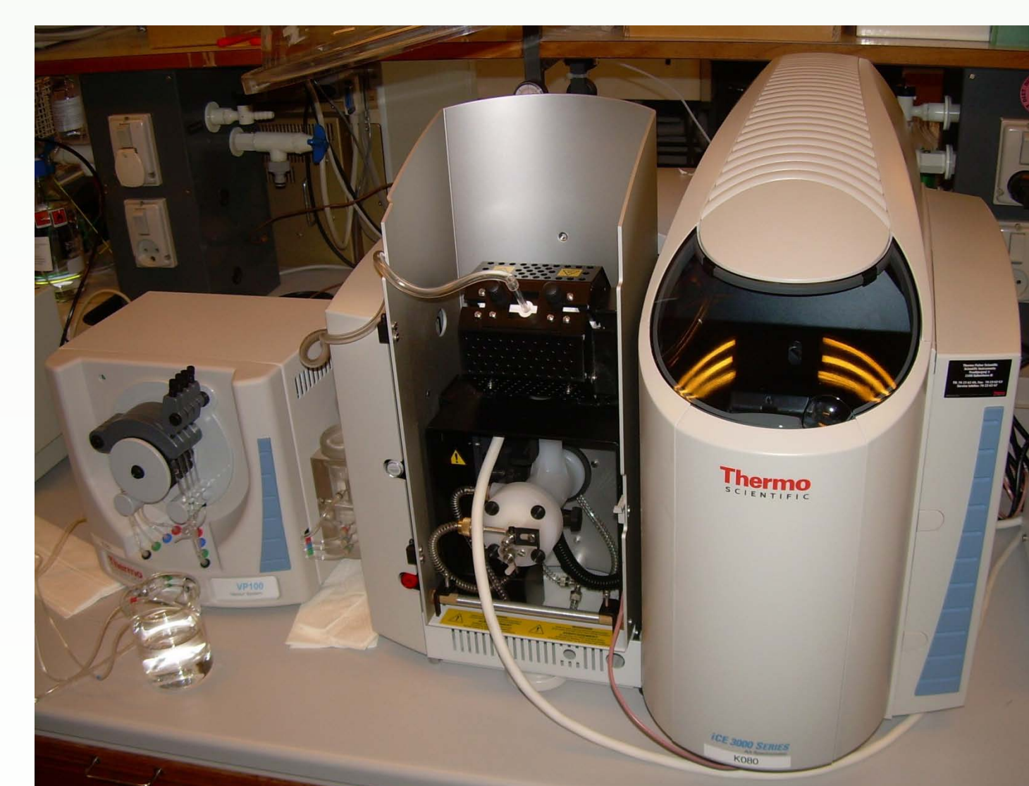
PICTURE 1. ICE 3300 AAS from Thermo Scientific with a VP100 for hydride generation system and an electrically heated cell.
